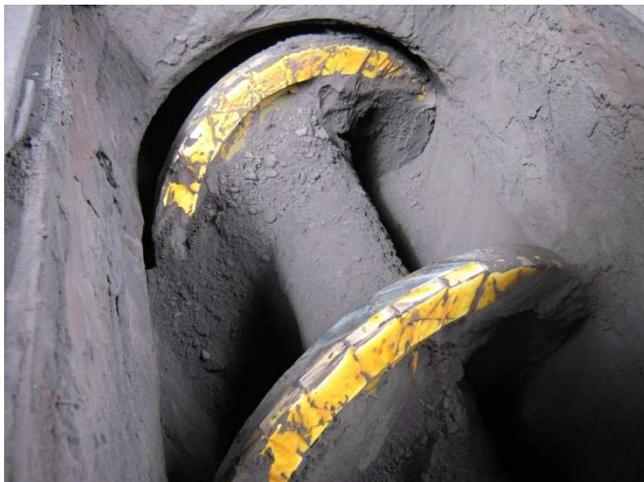
For this job Groupline protected one screw and after more than 3 years in operation, the screw is showing some signs of wear, but can still be used. The initial installation was also done to determine the following:
